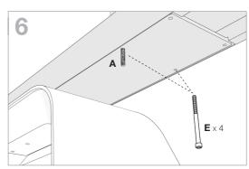
Secure with **(E)** on both sides, remove **(A)** and secure with remaining (E).
