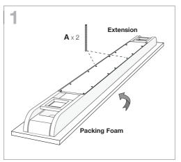
Carefully place extension on a soft surface/ packing foam. Screw on (A) diagonally on marked holes #1.
