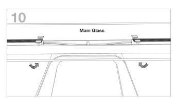
Once main glass is aligned, fully tighten (E) with allen key (I) shown in step 6.
