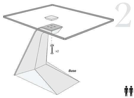
Using the threaded screws as guides, carefully place glass on base. Remove threaded screws once glass is aligned with base.
